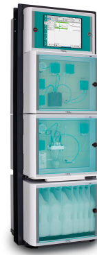
Figure 2. 2060 Process Analyzer from Metrohm for online monitoring of hydrogen peroxide during the CMP process.
