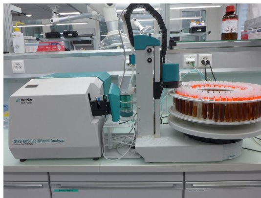
Figure 1. XDS RapidLiquid Analyzer with 5.0 mm flow cell and the 815 Sample Processor.
