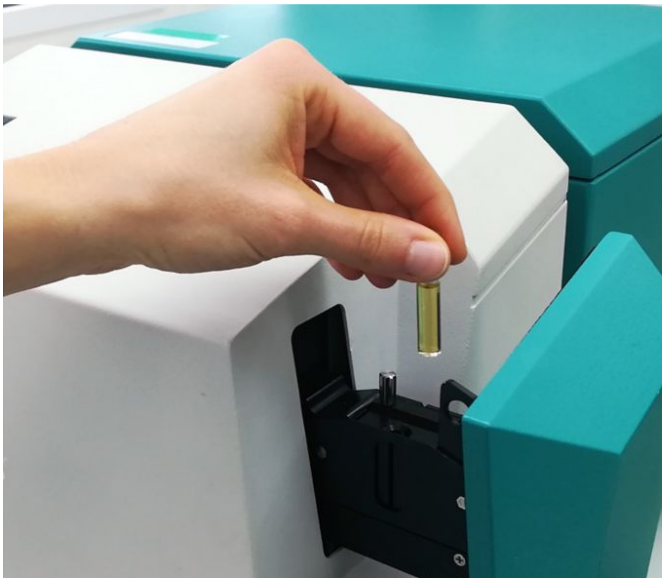
Figure 1. XDS RapidLiquid Analyzer and a palm oil sample present in a 8 mm disposable vial.
