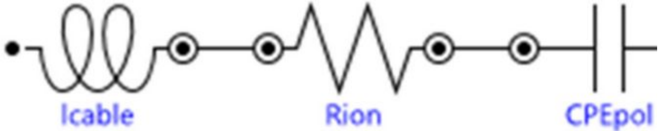
Figure 3. Equivalent circuit for fitting the impedance spectra.
