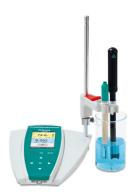
**Figure 1.** 914 pH/DO/Conductometer equipped with an O2-Lumitrode and conductivity sensor for the determination of dissolved oxygen in wine samples.
