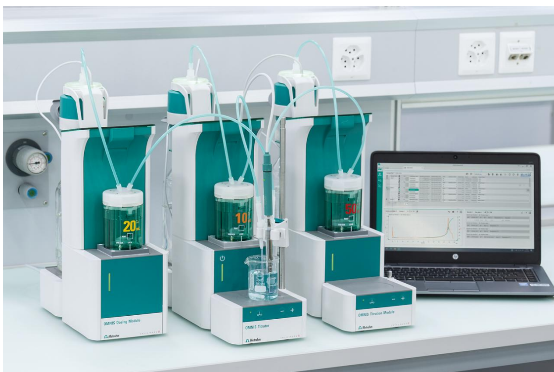
Figure 2. OMNIS Titrator equipped with a dSolvotrode electrode for the determination of caffeine content in nonaqueous samples.
