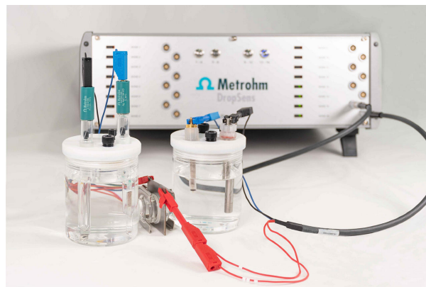
Figure 1. \mu Stat-i Multi16 instrument with H-CELL
