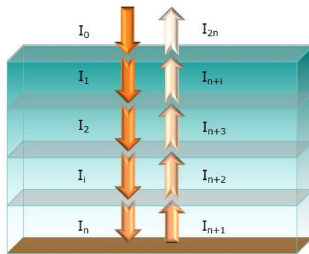
**Figure 2.** Normal reflection configuration.
