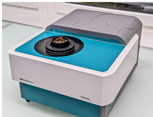
Figure 1. OMNIS NIR Analyzer Solid with roasted coffee beans in the small cup OMNIS NIR, 60 mm.
