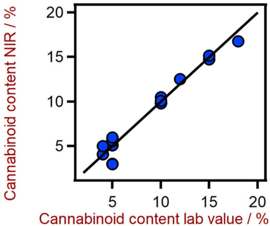
**Figure 3.** Correlation diagram for the prediction of cannabinoid content in CBD oils using a DS2500 Liquid Analyzer.
