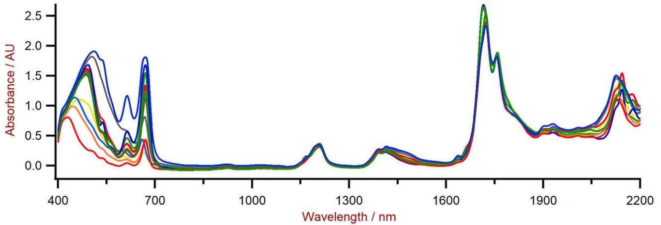
**Figure 2.** Vis-NIR spectra of CBD oils with varying cannabinoid content measured on a DS2500 Liquid Analyzer.
