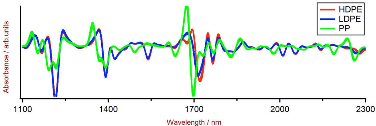
**Figure 2.** Selection of HDPE, LDPE, and PP NIR spectra (pre-treated with a 2nd derivative) obtained using a DS2500 Analyzer. Clear differences for the different polymer types are visible in the wavelength region around 1700 nm.
