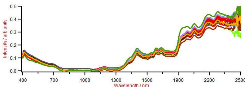
**Figure 2.** Protein samples measured with varying water content.
