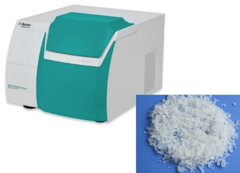
**Figure 1.** The DS2500 Solid Analyzer was used to collect the spectra of PVA polymer.
