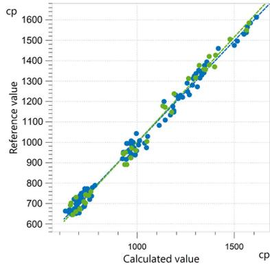
**Figure 5.** Correlation diagram and the respective FOMs for the prediction of viscosity of laundry detergent using an OMNIS NIR Analyzer Liquid. The correlation set is shown in blue, and the external validation set is in green. Reference values were obtained with a viscometer.
