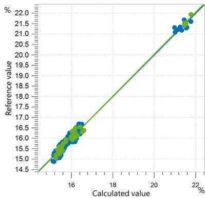
**Figure 4.** Correlation diagram and the respective FOMs for the prediction of dry matter in liquid laundry detergent using an OMNIS NIR Analyzer Liquid. The correlation set is shown in blue, and the external validation set is in green. Reference values were obtained via loss on drying.
