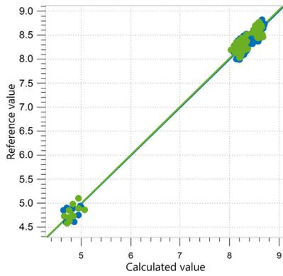
**Figure 3.** Correlation diagram and the respective FOMs for the prediction of pH value in liquid laundry detergent using an OMNIS NIR Analyzer Liquid. The correlation set is shown in blue, and the external validation set is in green. Reference values were obtained with a pH meter.
