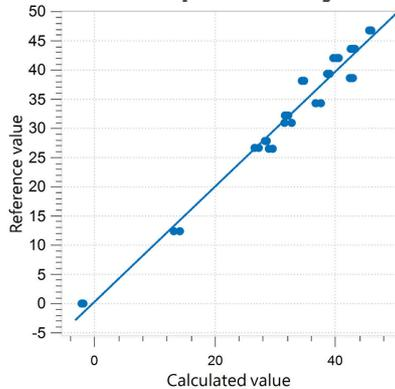
**Figure 6.** Correlation diagram and the respective FOMs for the prediction of surfactant content in liquid laundry detergent using an OMNIS NIR Analyzer Liquid. No external validation set was used. Reference values were obtained with potentiometric titration.
