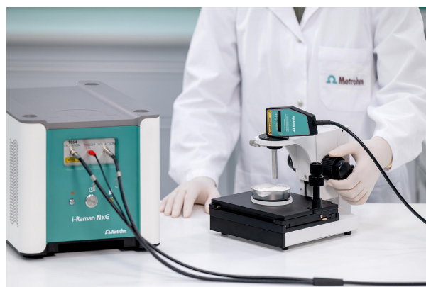
Figure 2. The i-Raman NxG 1064 and mounted fiber-optic probe from Metrohm were used in this study.
