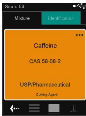
Figure 2. Actual screenshot of identification of caffeine in Yaba with MIRA DS. Caffeine is a chemical commonly associated with illicit drugs. The yellow warning background provides immediate, actionable information about the nature of the sample.
