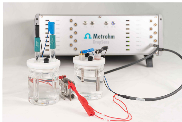
Figure 1. \mu Stat-i Multi16 instrument with H-CELL
