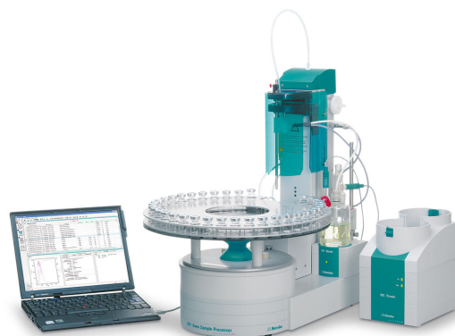
Figure 1. Fully automated system consisting of an 874 Oven Sample Processor with 851 Titrand for the coulometric Karl Fischer after vaporization of any moisture present in the sample.
