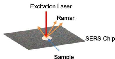
**Figure 1.** Illustration of a Raman Measurement Using a SERS Chip
