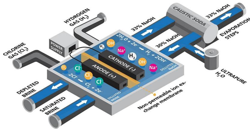
**Figure 1.** Diagram of the chlor-alkali membrane cell technique used to produce chlorine from saturated brine. Adapted from [www.eurochlor.org](http://www.eurochlor.org).
