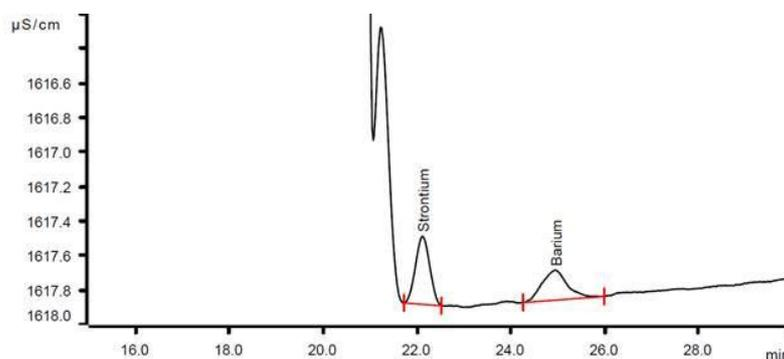
**Figure 3.** Chromatogram of a brine sample (>300 g/L NaCl) spiked with strontium and barium. A 4 mL sample aliquot was preconcentrated on the Metrosep Chel PCC 1 VHC/4.0 and then eluted on a Metrosep C6 separation column. The strontium and barium peaks are well separated from the large sodium matrix peak. Very low detection limits of multivalent cations in highly concentrated brines can be reached with this method.
