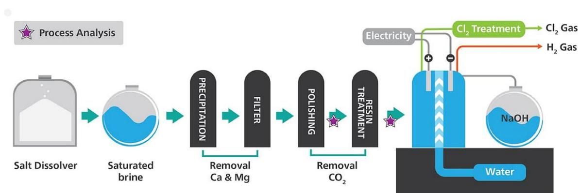
**Figure 2.** Schematic diagram of the overall chlor-alkali process with stars noting the ideal areas for online process analysis.
