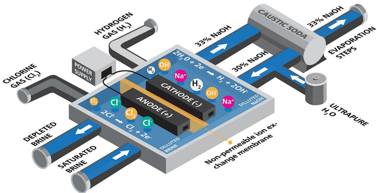
**Figure 1.** Diagram of membrane cell technique for the production of chlorine. Adapted from [www.eurochlor.org](http://www.eurochlor.org).
