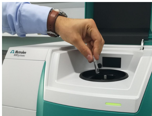
Figure 1. DS2500 Liquid Analyzer and a sample filled in a disposable vial.
