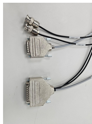
Figure 4. DIO trigger and BNC cable used in this system.
