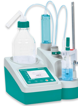
Figure 1. Eco Titrator equipped with a Ca-ISE electrode for the determination of Ca in aqueous solutions.
