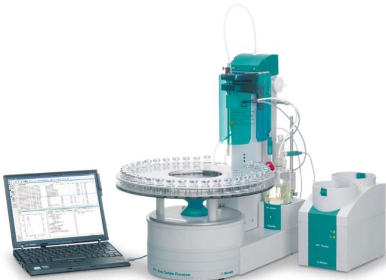
Figure 1. Fully automated system consisting of an 874 Oven Sample Processor with 851 Titrando for the coulometric Karl Fischer after vaporization of any moisture present in the sample.
