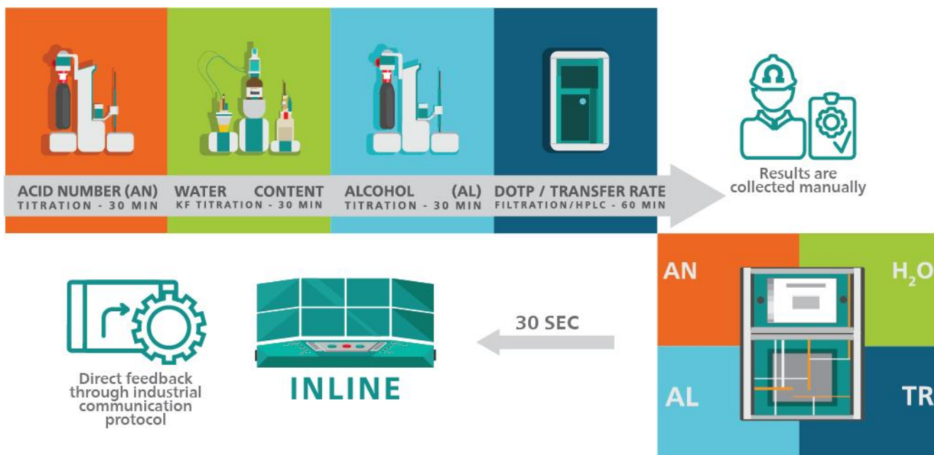
Figure 1. Steps to measure important parameters in DOTP production by implementing offline (top) or inline (bottom) analysis procedures.
