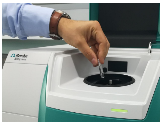
Figure 1. DS2500 Liquid Analyzer and a palm oil sample present in an 8 mm disposable vial.
