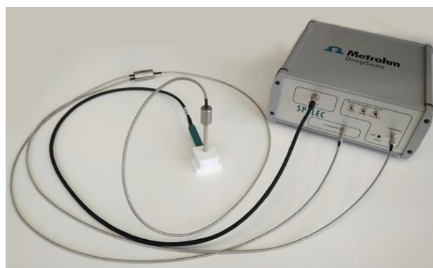
Figure 1. Setup for UV/VIS spectroelectrochemistry.
