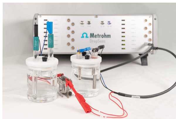
Figure 1. \mu Stat-i Multi16 instrument with H-CELL
