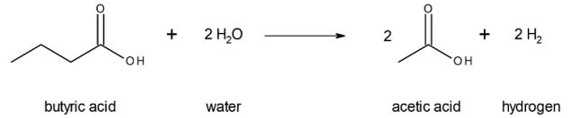
Equation 1: Chemical equation of the degradation process with butyric acid as example.
