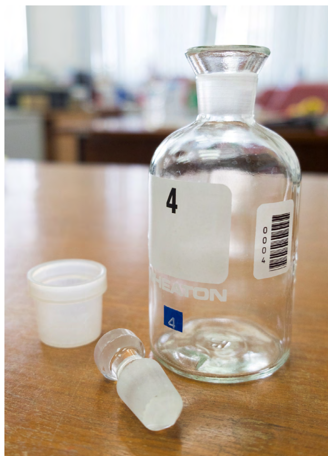
Figure 1. BOD bottle used for sampling ("Biological Oxygen Demand Bottle" by Mameaw.piti. CC BY-SA 4.0)
