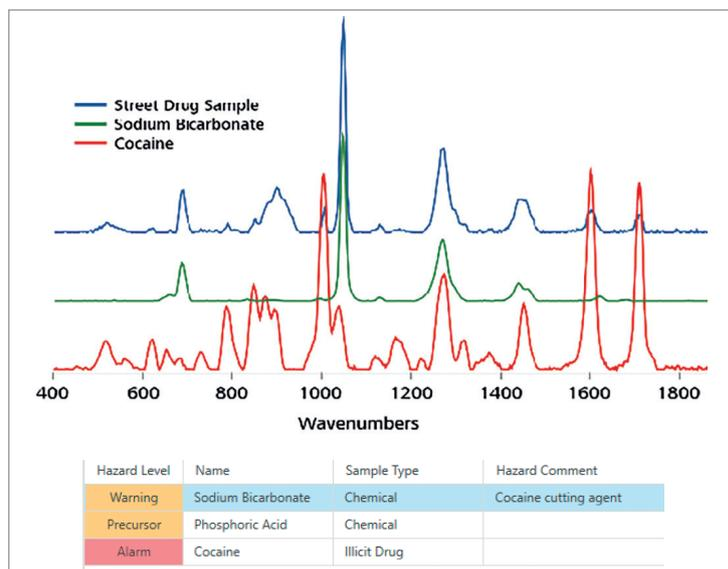
Figure 5. Sodium Bicarbonate is a Common Cutting Agent.
