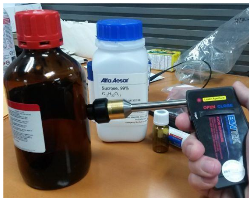
Figure 2: Focus Adaptor in place on the ST Probe
