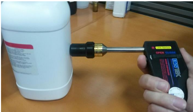
Figure 1: Focus Adaptor + Surface Regulator to Measure Package Material
