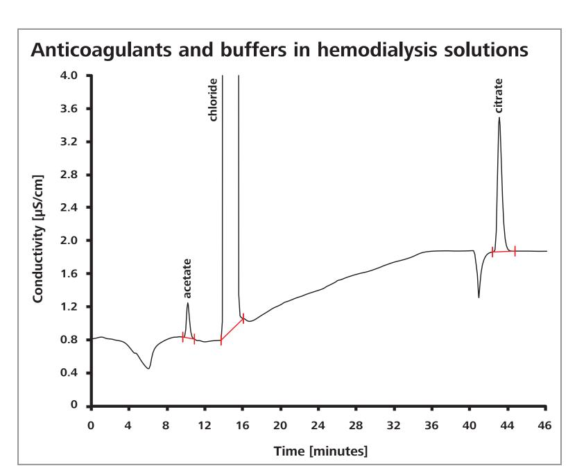
Acetate and citrate in diluted hemodialysis solution measured on a Metrosep A Supp 7 - 250/4.0 using a Na<sub>2</sub>CO<sub>3</sub>-gradient and conductivity detection after sequential suppression.
