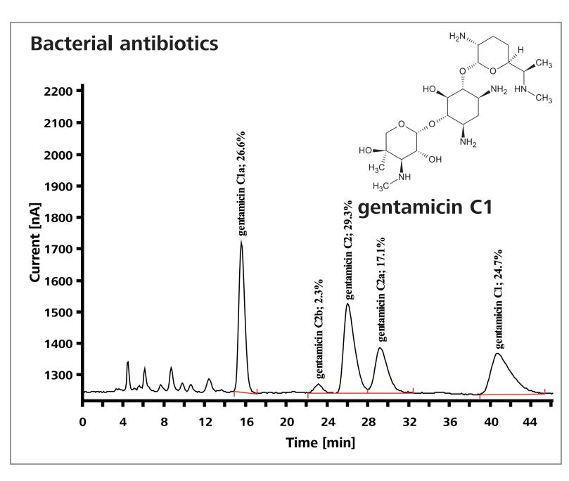
Separation of gentamicin analogs on a RP-S column (Polymer Laboratories) applying post-column addition of 300 mmol/L NaOH with pulsed amperometric detection (PAD).
