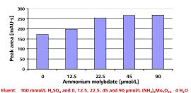
No significant enhancement in sensitivity was observed for concentrations exceeding 45  $\mu$ mol/L ammonium molybdate. Lower concentrations result in a loss of sensitivity. Without any molybdate ions the post column reaction proceeds to 70%.
