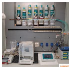
A sample assignment table ensures that samples with their own sample identification are automatically processed by the correct method. Repetitive identifications, such as occur in the preparation of external calibration standards, are saved in text templates and can be used again at a later date. For the preparation of a defined concentration of internal standard, automatic standard addition is carried out after previously weighing out the sample.
