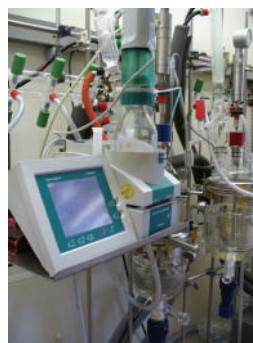
In the majority of applications, organo-magnesium and organo-lithium compounds and occasionally also silicium tetrachloride are added to carbonyl compounds. The dosing rates of the organo-metal compounds are in the range 0.1...2 mL/min; dosing times are from 2...5 hours.
