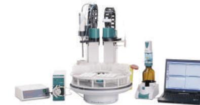
The tablets are automatically treated with eluent and then pulverized by a homogenizer. The resulting suspension is stirred for a few minutes before it is filtered through a disposable filter into a PP sample vessel or vial. The control of the dosing, filtering and sample changer operations, some of which are carried out in parallel, is by **tiamo™**, the laboratory automation and titration software.
