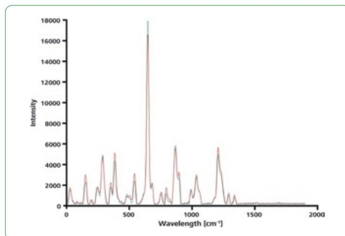
Fig. 4: This overlay of a single spectrum taken with ORS (green) and the average over 15 spectra measured without ORS (red) shows that the curves match nearly perfectly.
