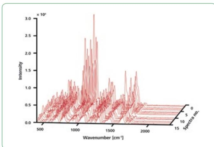
Fig. 2: The 15 Raman spectra shown here were recorded at random locations on a single sample without ORS. Although peaks are observed at the same positions, intensities vary.
