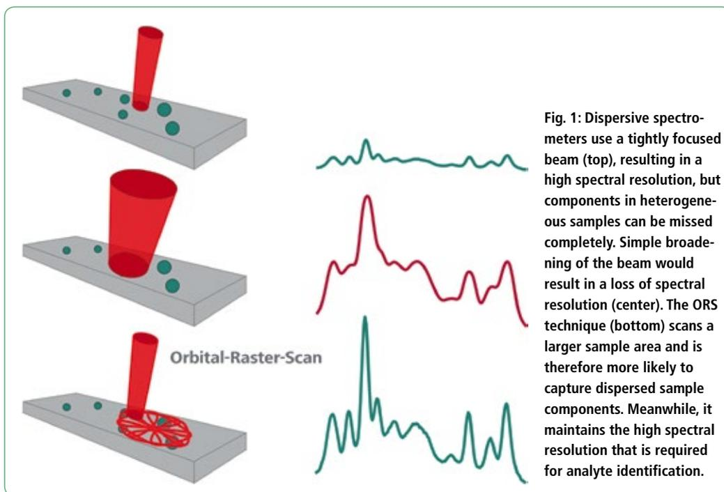
Fig. 1: Dispersive spectrometers use a tightly focused beam (top), resulting in a high spectral resolution, but components in heterogeneous samples can be missed completely. Simple broadening of the beam would result in a loss of spectral resolution (center). The ORS technique (bottom) scans a larger sample area and is therefore more likely to capture dispersed sample components. Meanwhile, it maintains the high spectral resolution that is required for analyte identification.
