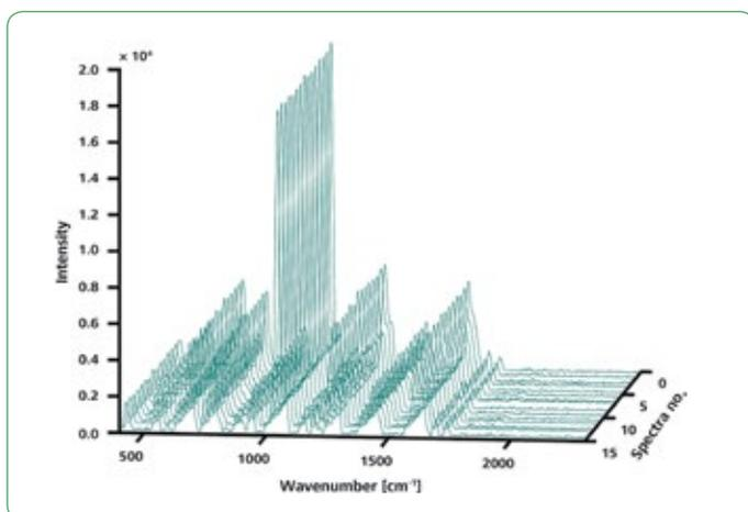
Fig. 3: Like in figure two, the 15 spectra shown here were measured at random locations on a single sample. However, in this measurement, ORS was used sampling an area of 3 mm diameter. The spectra are visibly congruent.
