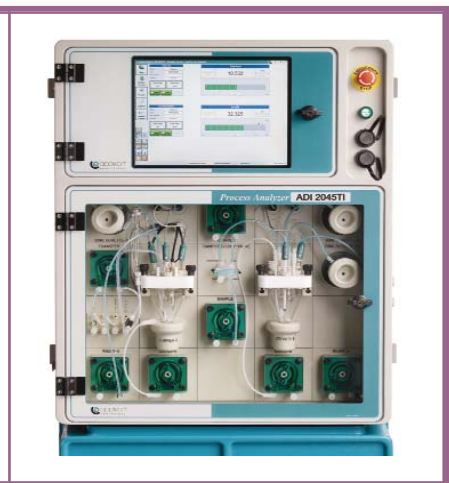
Figures 5 & 5a. Rendering of an analyzer that is closely integrated with the plating process
