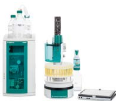
Figure 1. The experimental setup consists of an 881 Compact IC pro with the 858 Professional IC Sample Processor with dialysis cell and 800 Dosino. Instrument control, data acquisition and processing were carried out by MagIC Net software.
