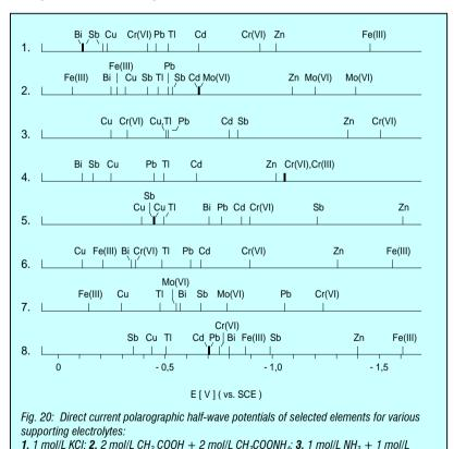
$NH_aCl$ ; **4.** 1 mol/L HCl; **5.** 1 mol/L NaOH; **6.** 0.5 mol/L Na-tartrate; **7.** 0.1 mol/L  $Na_2$ -EDTA; **8.** 1 mol/L Na-citrate + 0.1 mol/L NaOH (measured against the saturated calomel electrode)
