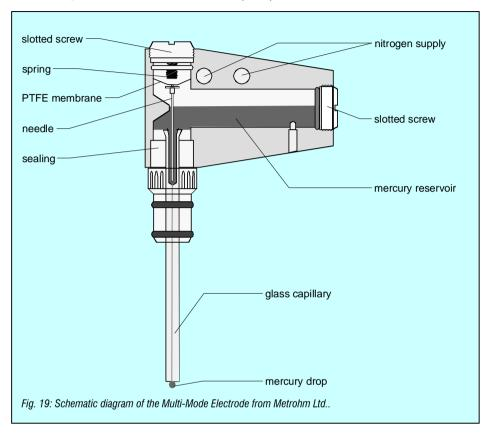
In the Multi-Mode Electrode the mercury is controlled pneumatically via a needle valve; the inner diameter of the capillary is about 50  $\mu$ m. Small mercury drops with a surface area of 0.1 to 0.6 mm² are generated (can be set in 9 steps), with which in ASV determinations similarly narrow peaks can be obtained to those produced by mercury film electrodes.
