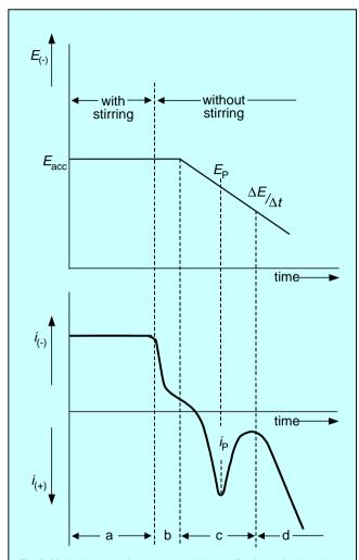
Fig. 8: Method steps and current-potential curve for determinations by anodic stripping voltammetry
