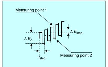
Fig. 5: Measuring technique of square wave voltammetry acc. to Osteryoung  $\mathbf{t}_{step}$  Duration of a potential step or a square wave pulse (10 ms);  $\Delta \mathbf{E}_{A}$  Square wave potential amplitude (20 mV);  $\Delta \mathbf{E}_{step}$  Potential step of the staircase ramp (4 mV)
