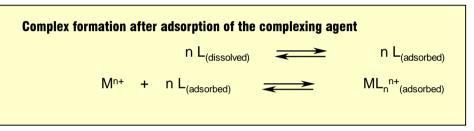
3. If M<sup>n+</sup> does not form a surface-active compound with the complexing agent, the analyte will be electrochemically reduced or oxidized and transformed into a suitable oxidation state for complex formation. The process takes place either in the solution or on the electrode surface.
