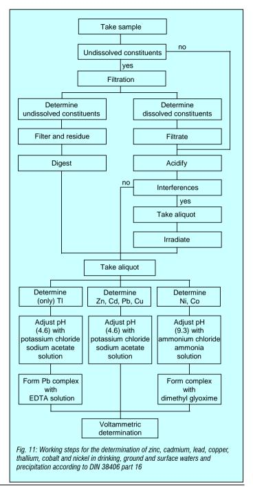
Chemical digestions are necessary for the ASV determinations of traces of metals in strongly polluted water (e.g. in wastewater). Oxidizing wet-chemical digestions in a flask fitted with a reflux condenser and absorption vessel or in a Digesdahl digestion apparatus are most frequently carried out (digestion as per DIN 38414 part 2 (1983) and part 7 (1982)). The same applies for the digestion of sewage sludge, soils and sediments.
