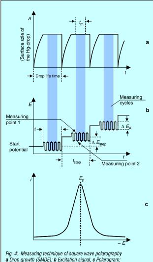
Fig. 4: Measuring technique of square wave polarography a Drop growth (SMDE); **b** Excitation signal; **c** Polarogram;  $\Delta E_{step}$  Potential step for staircase ramp (up to 2-12 mV);  $t_{step}$  Duration of a potential step (0.5-10 s);  $\Delta E_A$  Square wave potential amplitude ( $\sim 25$  mV);  $t_m$  Measuring time; **f** Oscillation frequency (approx. 125 Hz for t = 40 ms)
