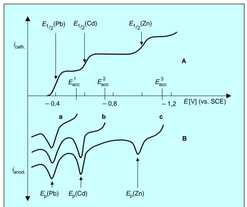
Fig. 9: Principle of selective and simultaneous ASV determination of lead, cadmium and zinc **A** DC polarogram of Pb, Cd and Zn (each  $10^{-3}$  mol/L) in 0.1 mol/L KCl; **B** Stripping voltammogram of Pb, Cd and Zn (each  $10^{-5}$  mol/L) in 0.1 mol/L KCl after accumulation at different potentials; **a**  $E^1_{acc}$  for lead; **b**  $E^2_{acc}$  for lead and cadmium; **c**  $E^3_{acc}$  for lead, cadmium and zinc
