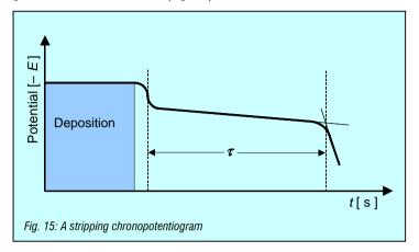
Accumulation takes place at a constant potential and for a controlled time at a mercury, glassy carbon or platinum electrode in a stirred sample solution. Mercury films are normally used for deposition of metals, these are applied to a graphite support by the *in situ* or *precoating* method.
