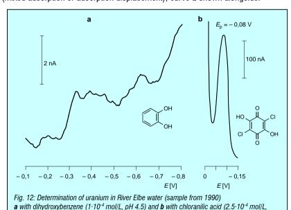
pH 2.7) as complexing agent and after accumulation at  $E_{acc} = +100 \text{ mV}$
