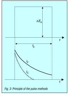
The methods developed with square wave potential pulses differ in the frequency and height (amplitude) of the applied pulses as well as in the formation principle of the measured value. All methods can be carried out polarographically with the static mercury drop electrode or voltammetrically with stationary mercury electrodes or with solid-state electrodes.
