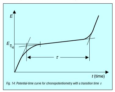
The two time sectors in which the potential increases relatively quickly are characteristic for the potential-time curve. From an analytical point of view it is the time between them (known as the *transition time*  $\tau$ ) that is important; at a constant current density j (current intensity i per electrode surface area A in the units A/cm²) it is proportional to the concentration of the analyte.
