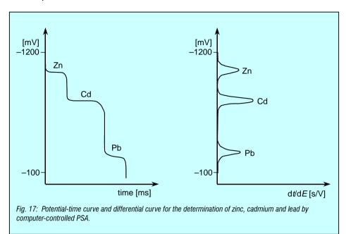
As the interference from organic contaminants in the trace analysis of elements by stripping chronopotentiometry is less then in stripping voltammetric determinations, UV or microwave treatment of aqueous samples is not always necessary. It is often sufficient if the strongly polluted water samples are diluted before analysis. Degassing is also unnecessary, as the dissolved oxygen is required for the oxidation of the accumulated analyte.
