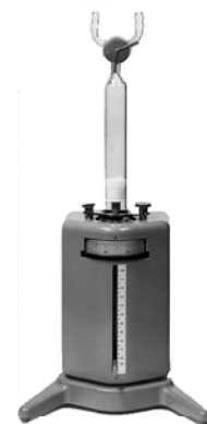
First piston buret (Metrohm 1955) PTFE piston in a calibrated glass tube. Highly accurate volume resolution according to the micrometer principle.
