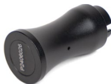
Figure 18: Performance Validation Cap for Raman probes with a shaft diameter of 9.5 mm
