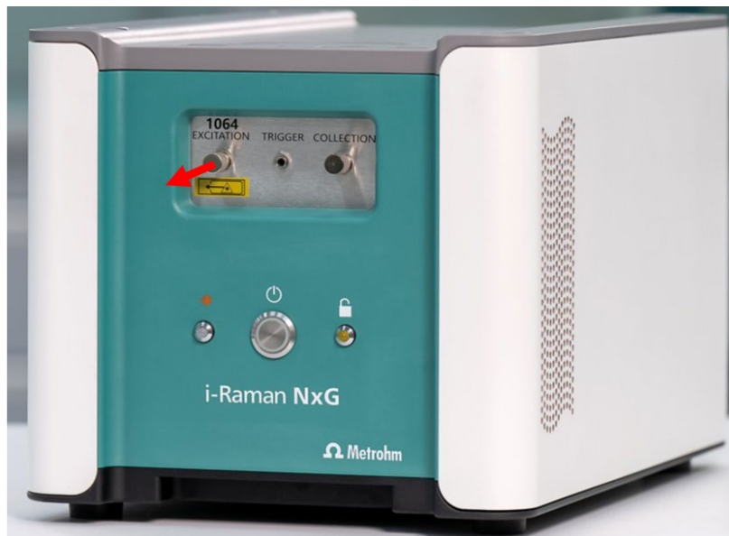
Figure 3: System laser emission aperture with fiber disconnected
