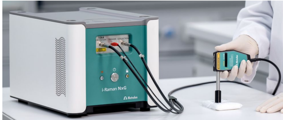
Figure 13: Scanning with the distance regulator
