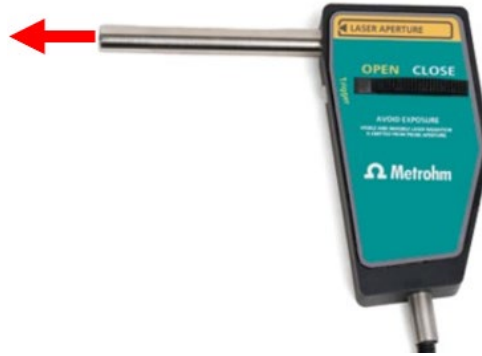
Figure 2: Raman Probe laser emission aperture
