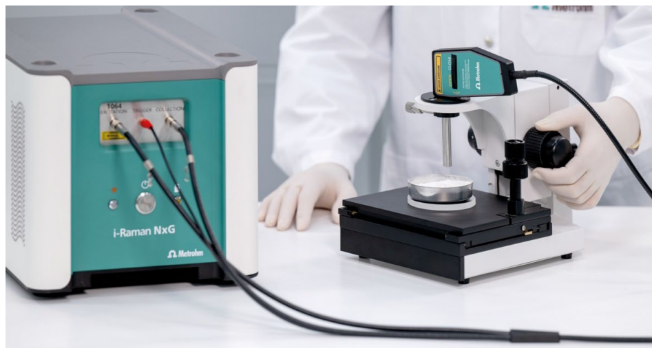
Figure 14: Fine adjusting the sampling position with Raman probe holder
