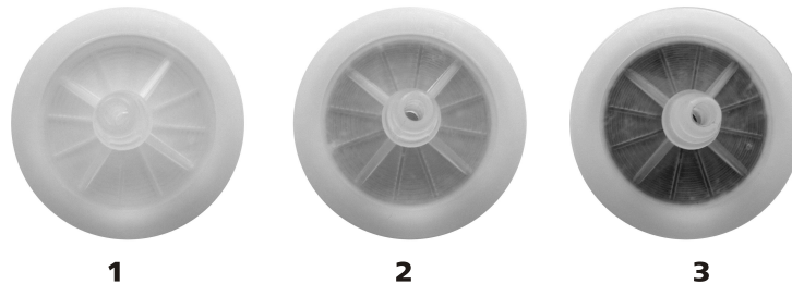
Figure 17 Dust filter - conditions
