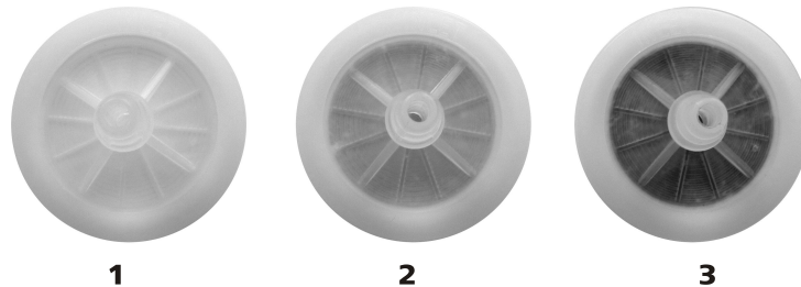
Figure 18 Dust filter - conditions
