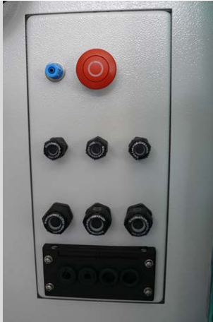
Figure 11: Compressed air line connector
