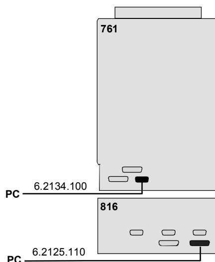
Figure 5: Connecting the 816 IC Eluent Selector to a PC
