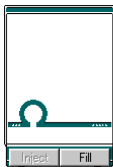
System connected Injection valve in "INJECT" position
