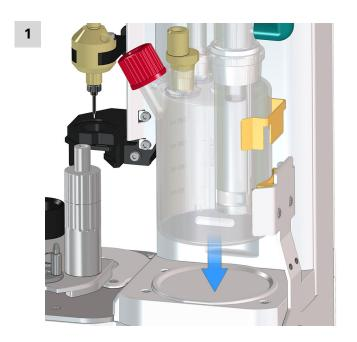
Insert the metal clip on the Karl Fischer titration cell into the titration vessel holder.
