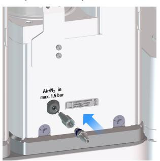
If gas is fed from a pressure line or a pressure vessel, then an upstream pressure reduction valve must be installed. The input pressure must be set with the valve closed and must not exceed 1.5 bar of overpressure. The nominal operating pressure is 1.0 bar.
