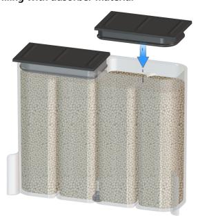
• Fill the adsorber cartridge with adsorber material up to the ridge height. A wad of cotton is not required as there are filters in the suction stoppers.
