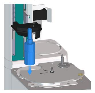
• Loosen the adjustment pin (5-4) and the centering disk.
