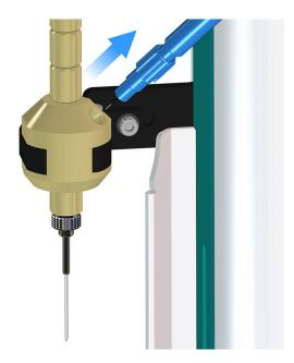
■ Loosen and remove the FEP tubing (7-9).
