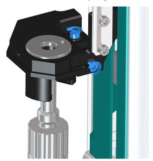
• Lower the vial holder (7-4) and align it to the centering disk (5-4) by moving the needle holder (7-8) along the x- and y-axes.
