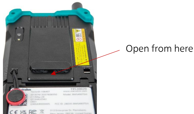
Figure 19: How to remove the back fan
